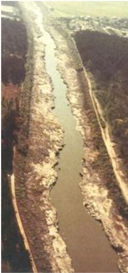
River bed erosion and bank erosion\*
